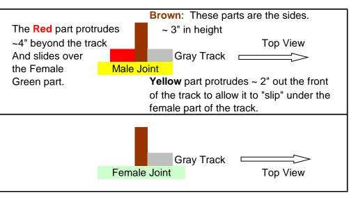
Top drawing is the Male part of the track. This end SIDE VIEW points down the hill. ~15 & 7/8" inside width. \_ Drawing below is the Female part of the track. This end points up the hill. SIDE VIEW Track continues When the two joints come together, the red tabs go on top of the green part. The yellow section goes under the track part below. Red tabs centers track joints to ensure the sides do not stick out.
